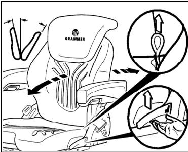
Pull up the locking lever to release the backrest catch.
