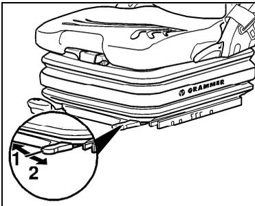
The fore/aft isolator improves the absorption of shock impacts (e.g. when driving at high speed, in rough terrain or with a trailer attached) in the driving direction by the driver's seat.
